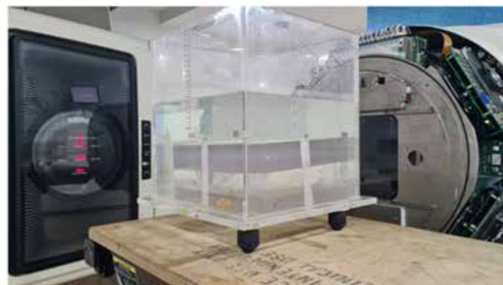
Fig. 1: ECRT set-up with a water phantom customised as bone irradiator
