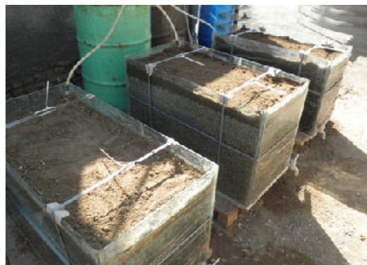
Fig. 1: Glass pilot plant of subsurface flow wetland
