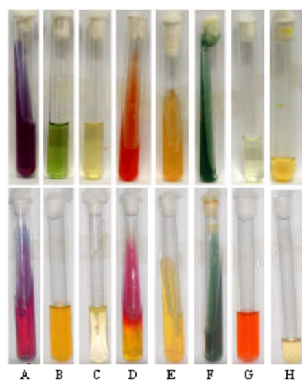
Fig1: Differential and selective media used for the detection of Salmonella enteritidis in poultry products. The tubes are before inoculation media. A: lysine, B: phenylalanine, C: SIM, D: TSI, E: urea, F: cimon citrate, G: MR and H: VP
