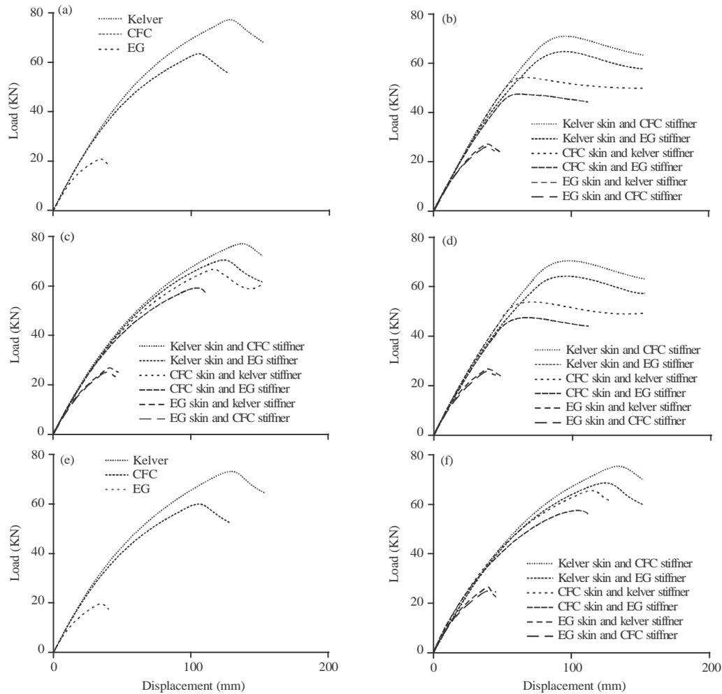
Fig. 6(a-f): Variation of the loads buckling as function displacement with the different layup sequences and combinations of composite material, (a) Layup sequence (45/-45/90/0)<sub>s</sub>; (b) Layup sequence (45/-90/0)<sub>s</sub>; (c) Layup sequence (90/0/90/0)<sub>s</sub>; (d) Layup sequence (90/0/90/0)<sub>s</sub>; (e) Layup sequence (60/-30/90/0)<sub>s</sub> and (f) Layup sequence (60/30/90/0)<sub>s</sub>
