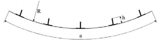
Fig. 1: Panel cross-section
