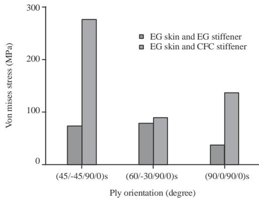
Fig. 8: Von Mises stresses obtained for the various ply layout sequences
