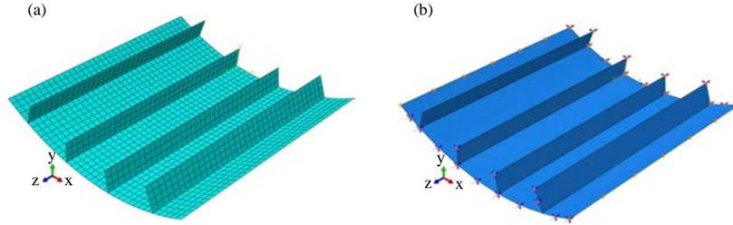
Fig. 4(a, b): (a) Finite element models with the straight stiffeners (b) and Finite element model with configuration boundary conditions and loads
