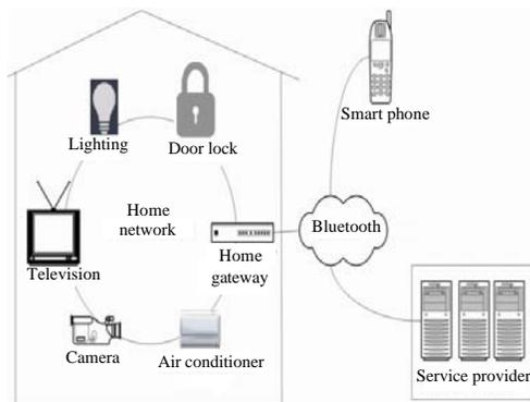
Fig. 6: SHAS-IoT systems diagram
