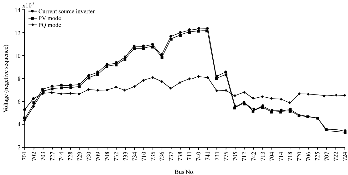
Fig. 10: Negative sequence voltage profile of 37 bus network with a 900 kW DG installed at bus 738 (for 3 cases: operating as a PV bus as PQ bus and as a partial unbalance compensator)
