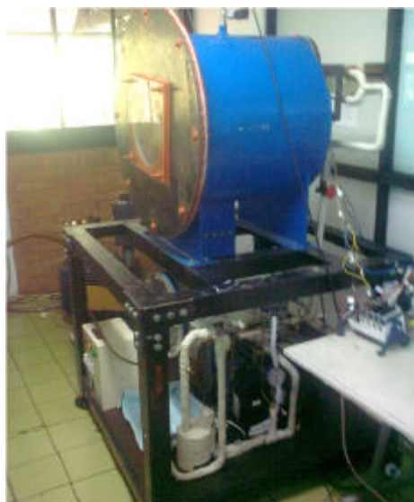
Fig. 2: Freeze vacuum drying system with heat source from heat loss condenser
