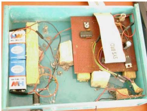
Fig. 2: A prototype Basal Body Temperature (BBT) logger
