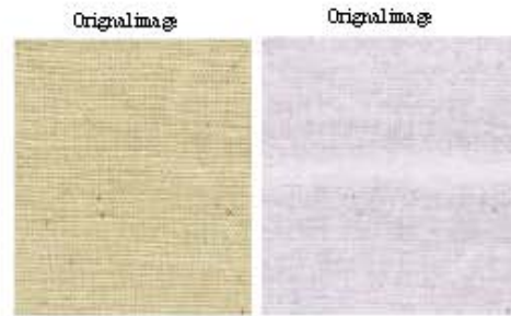
Fig. 3: Original flawless sample used for comparison in the detection of missing yam class of defects
