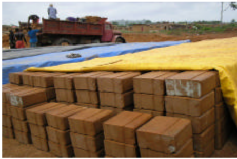
Plate 1: Stacked solid interlocking blocks in obasarjo's housing estate, Ado-Ekiti. Source: Field Survey (2007)
