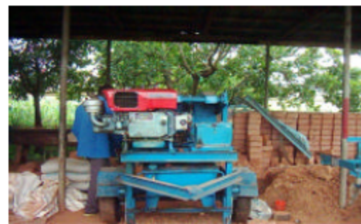
Fig. 2: Interlocking machine developed by NBRRI, Ota. Source: Researcher's field survey (2005), Ondo State housing corporation, Akure
