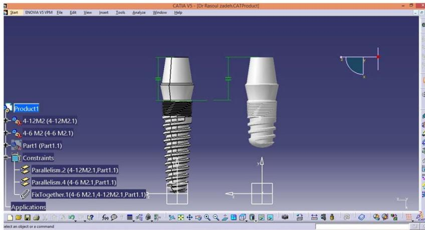
Fig. 1: Modeled implants with 5 mm long abutments with a micro-thread coronal surface and a tapered macro-thread body with equal 4 mm diameters and variable lengths
