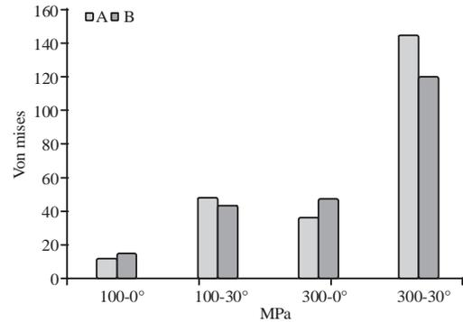
Fig. 4: The stress concentrated in cortical bone due to the application of different loads
