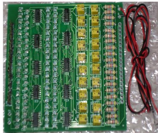
Fig. 6: Eagle 2-layer finished board top (left) after assembling
