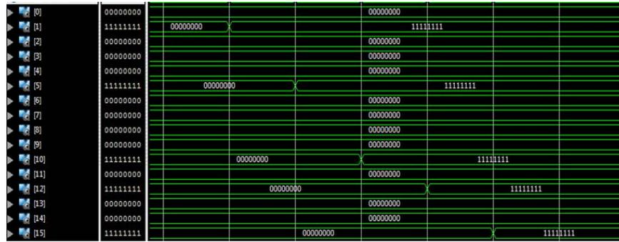
Fig. 15: Message (11111111) is transmitted along the selected path (1->5->10->12->15)
