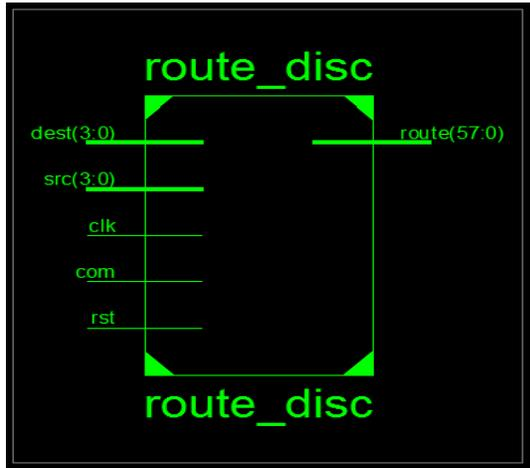
Fig. 5: Black box representation of the main controller
