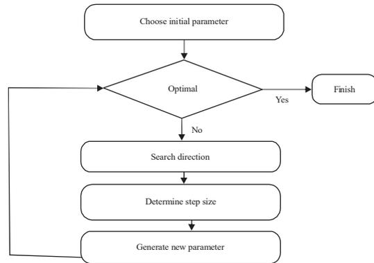
Fig. 5: Flow diagram of gradient descent algorithm
