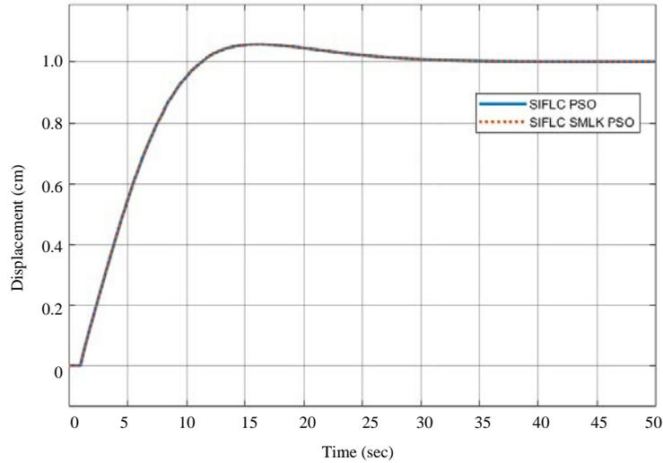
Fig. 7: Comparison result between PSO result using command windows (SIFLC PSO) and Simulink (SIFLC PSO1)
