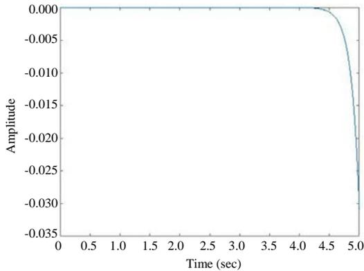
Fig. 4: Open loop step response of the rotational pendulum (1 volt step input)
