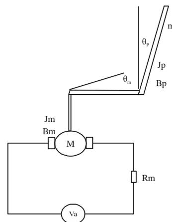
Fig. 1: Rotational pendulum
