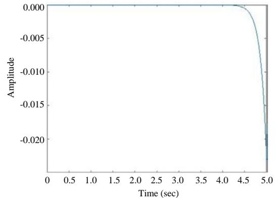
Fig. 3: Open loop impulse response of the rotational pendulum (1 volt impulse input)
