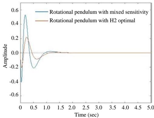
Fig. 5: Impulse response of the rotational pendulum (1 volt impulse input)
