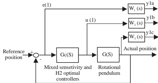
Fig. 2: Weighted control structure with the proposed controllers
