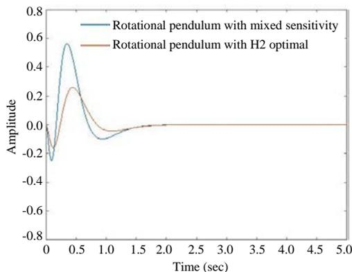
Fig. 6: Step response of the rotational pendulum (1 volt step input)
