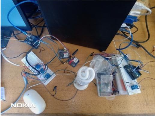
Fig. 3: The implementation model for the smart microgrid power pool system
