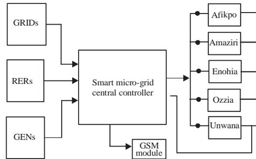
Fig. 1: The block representation of the smart microgrid power pool system
