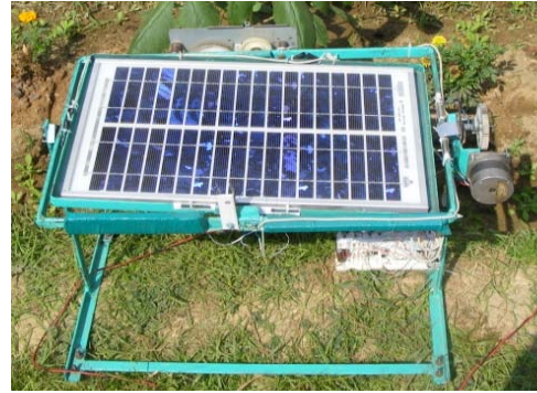
Fig. 10: Laboratory prototype of hybrid solar tracker
