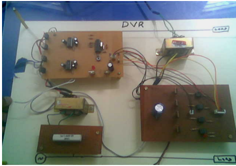
Fig. 12: Laboratory model of DVR system
