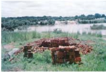
Fig. 7: Loam pit for bricks at the edge of the Milo River in Kankan widening the bed of the river
