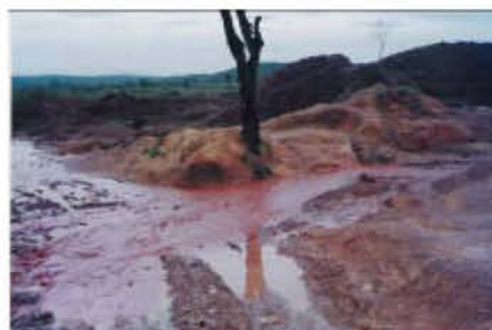
Fig. 2: Diamond mining site from Foulifimba (Sonaferiya) Banankoro to Kerouane; lack of rehabilitation of the grounds has contributed to the vast level of soil erosion
