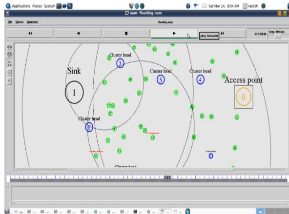
Fig. 12: Detection of flooding attacker node in nam window
