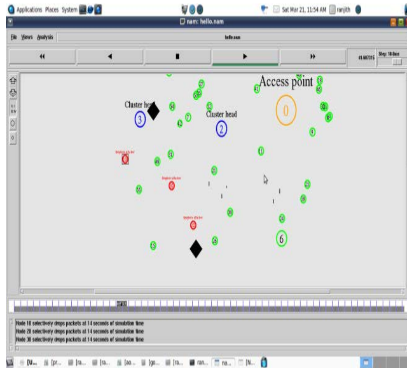
Fig. 14: Detection of gray hole attacker in Nam window
