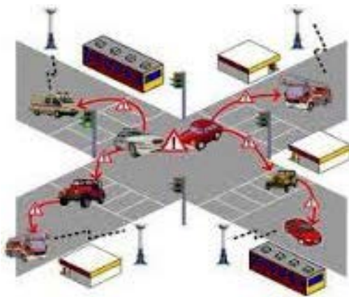
Fig. 2: Rout map based detection procedure of Sybil attacks in VANETS
