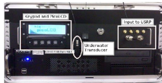
Fig. 2: Front view of UANT system
