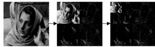
Fig. 3: Wavelet decomposition (I and II stage)
